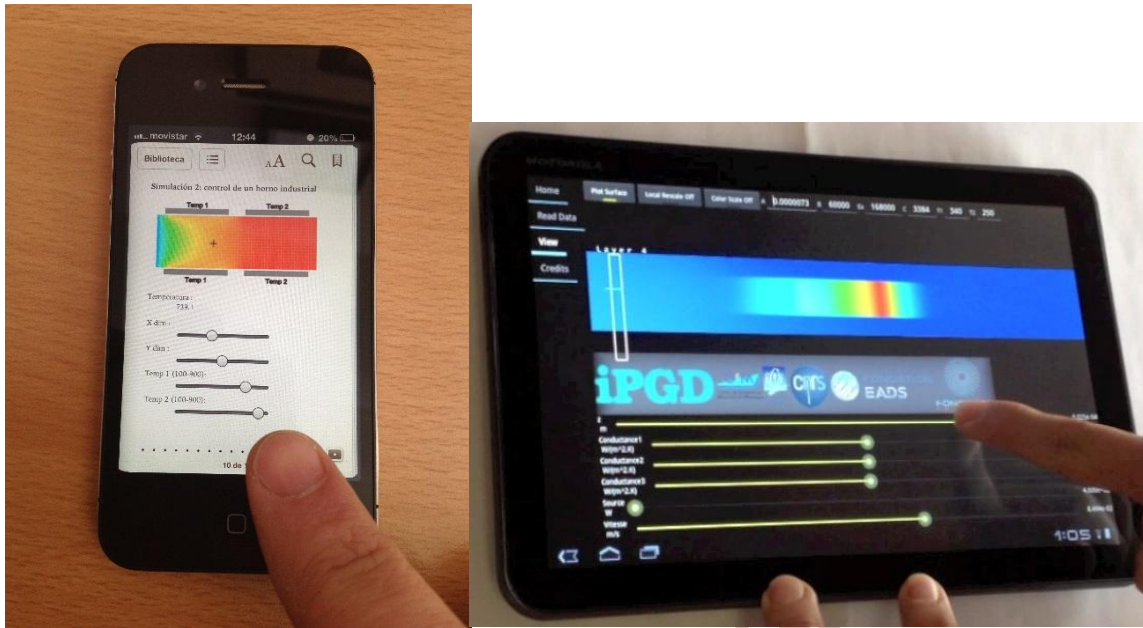
Figure 13. Exploring a PGD Computational Vademecum on a smartphone (left) and on a tablet (right).
