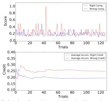
Fig. 3. At the top: Score evolution at each trial for each candidate network  $N \in \mathcal{N}$ . At the bottom: Average accumulated credits for right and wrong components. The simulation is done using a set of candidates *C* composed of n = 8 components. The average accumulated right credit (resp. wrong credit) was computed using an element belonging to the target (resp. does not belonging to the target).
