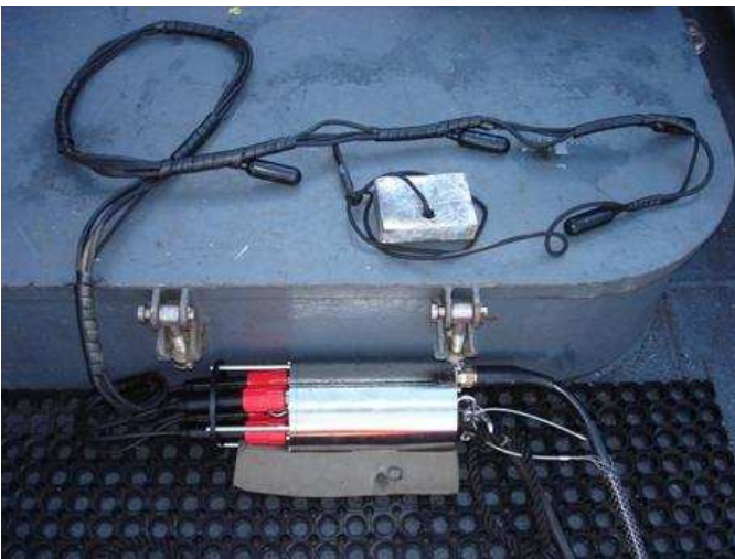
Fig. 9. The four hydrophones of the receiver
