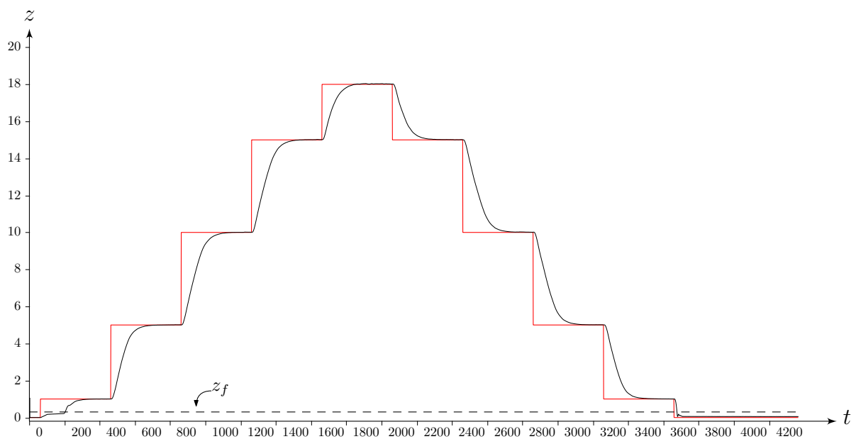
Figure 7: Depth z (in meter) of the float in function of time t (in seconds). The setpoint trajectory is in red and the float trajectory is in black.
