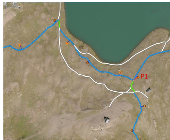
Figure 2. Map-matched GPS points (orange) to the BDTopo road network (blue). The point P1 is matched with the nodes to maintain consistency of the route.
