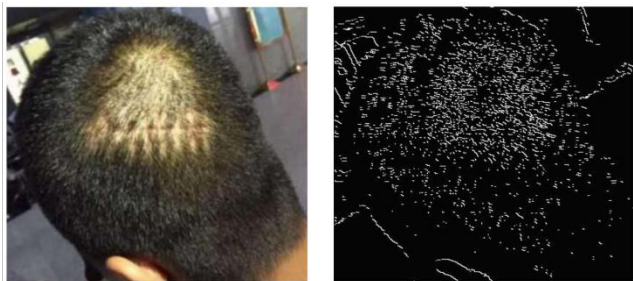
Figure 5. The original image (left) and the output (right) of the Canny algorithm.
