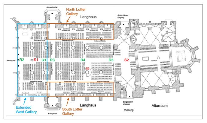
Figure 1. Plan of Thomaskirche, with positions of Lotter galleries and source/receiver positions during impulse response measurements.
