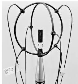
Figure 1. Custom microphone array (5 cm radius).
