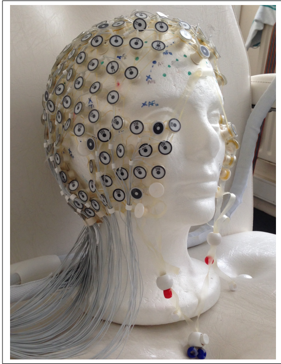
Figure 1. EGI sensor net composed of 256 electrodes.
