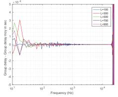
**Figure 7**. Deviations from the ideal group delays, for different lengths of sectioned convolutions.
