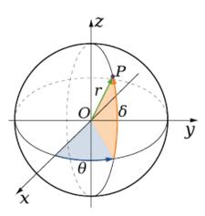
**Figure 1**. Spherical coordinate system. A point P (x, y, z) is described by the radius r, azimuth  $\theta$  and elevation  $\delta$ .
