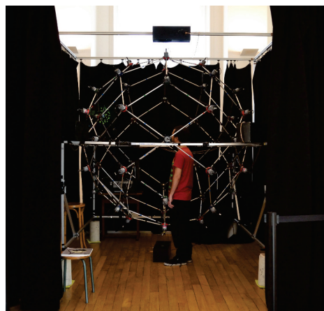
Figure 9. Cnam prototype of 5th order ambisonic restitution sphere.
