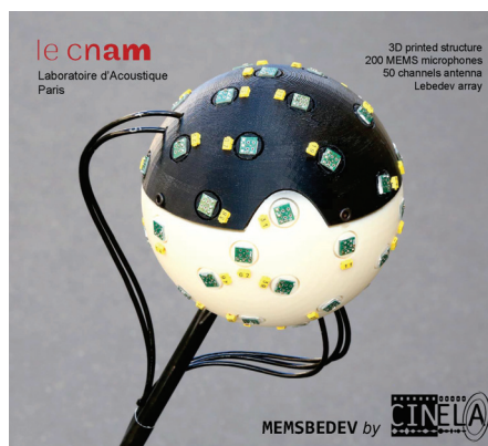
Figure 8. Cnam prototype of 5th order ambisonic recording sphere.
