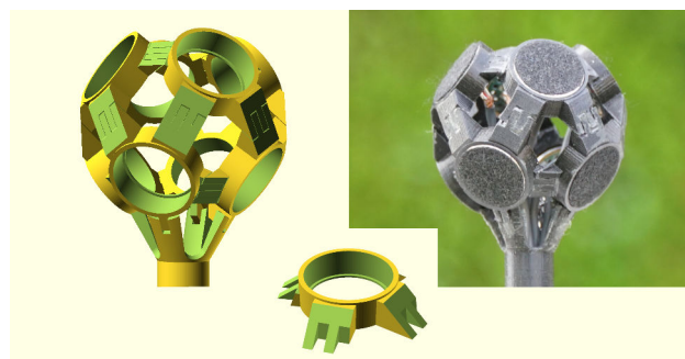
Figure 2. OctaSpHEAR v1 capsule array and individual capsule holder
