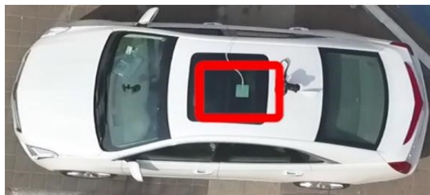
Figure 2: External microphone array on the roof of the car.
