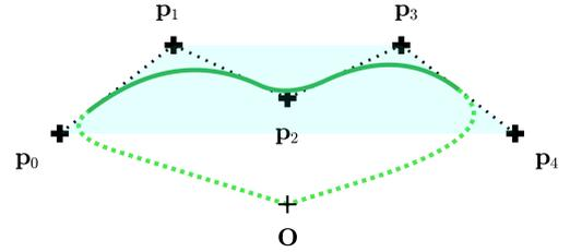
Figure 3: Convex hull of a B-spline of degree 2
