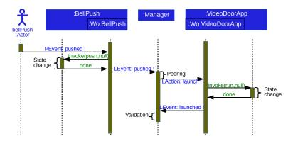
${\bf Fig.\,10.}$  UML Sequence diagram of the interaction between a physical bell push and a logical video application [2]
