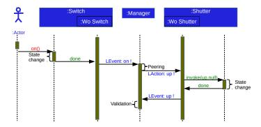
**Fig. 3.** UML Sequence diagram of the interaction between a WO switch and a WO shutter [2]
