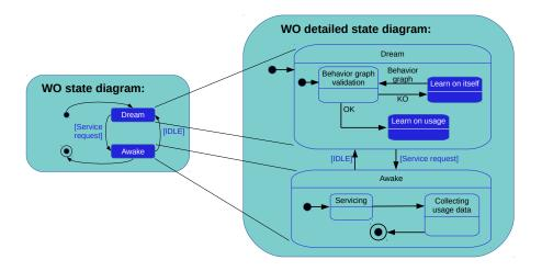
Fig. 4. UML state diagram of WO built-in behavior [4]
