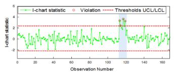
Fig. 10. Time evolution of the Shewhartl-chart statistic in the presence of an abnormal situation (Case  $A_1$ ).
