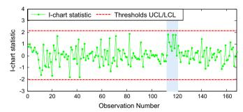
Fig. 13. Time evolution of the I-chart statistic in the presence of an abnormal situation (Case  $A_2$ ).
