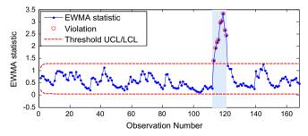
**Fig. 12.** Time evolution of the EWMA statistic in the presence of an abnormal situation (Case  $A_1$ ).
