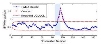
**Fig. 18.** Time evolution of the EWMA statistic in the presence of a gradual abnormal situation
