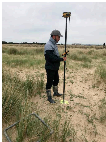
Figure 2. Ground control point acquisition using a DGNSS.
