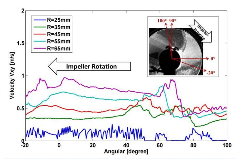
Highlight 1: PIV has been applied to study local velocity in a specific dynamic filtration module.
