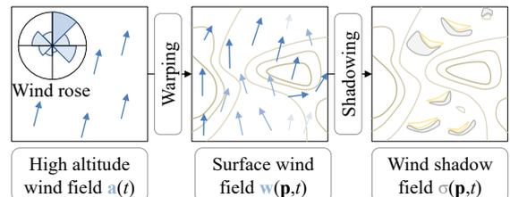
**Figure 4:** Overview of the wind field computation.
