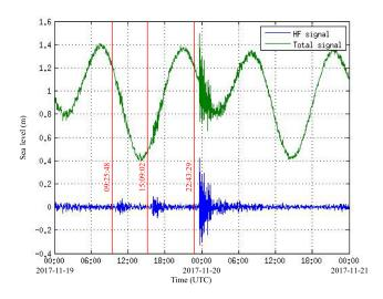
**Figure 8.** The triplet of tsunamis of 19 November 2017 recorded by the Ouinné tide gauge. The blue graph shows the filtered signal without the tide (the tide signal is visible on the green graph). The red lines show the times of the three different earthquakes.
