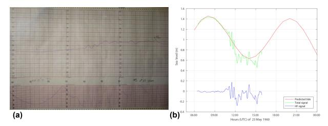
Figure 11. Tide gauge record of the 22 May 1960 Chile tsunami in Nouméa (Chaleix station): original record (a) and digitized signal (b), total (in green) and detided (in blue).
