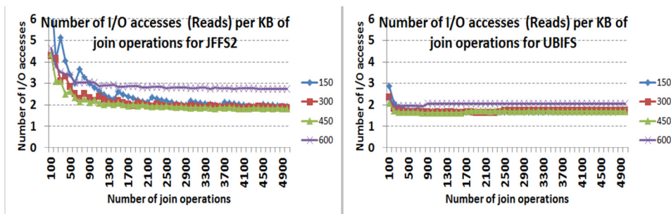
Figure 8: Number of I/O accesses to the flash memory for join operations according to record size and number of requests
