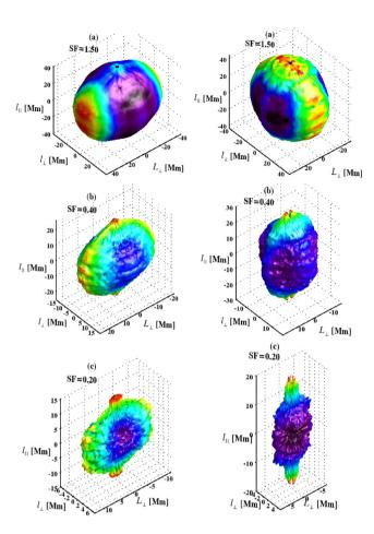
**Figure 11.** Strong-expansion data set (left) and weak-expansion data set (right). Isosurface of constant energy of the velocity structure function at three different levels,  $SF \approx 1.5, 0.4, 0.2$ , in panels (a), (b), and (c), respectively. The colour is redundant, it indicates the distance from the centre for better visualization.
