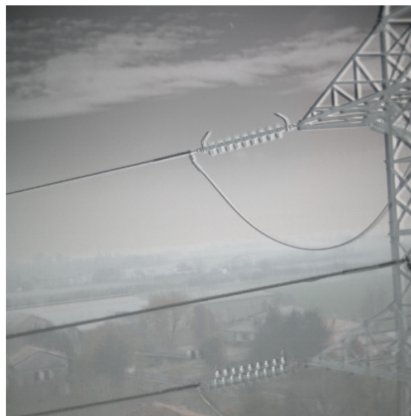
Figure 7. Overlapping of fixed (visible) and moving (IR) images with same size after registration.
