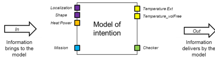
Figure 4: A blank model of intention with different port type (color) associated to attributes (name)
