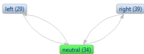
Figure 6: Allowed Transitions for Steering
