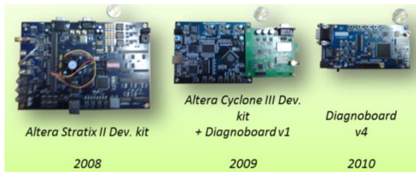
Figure 3: Reflectometry electronic boards
