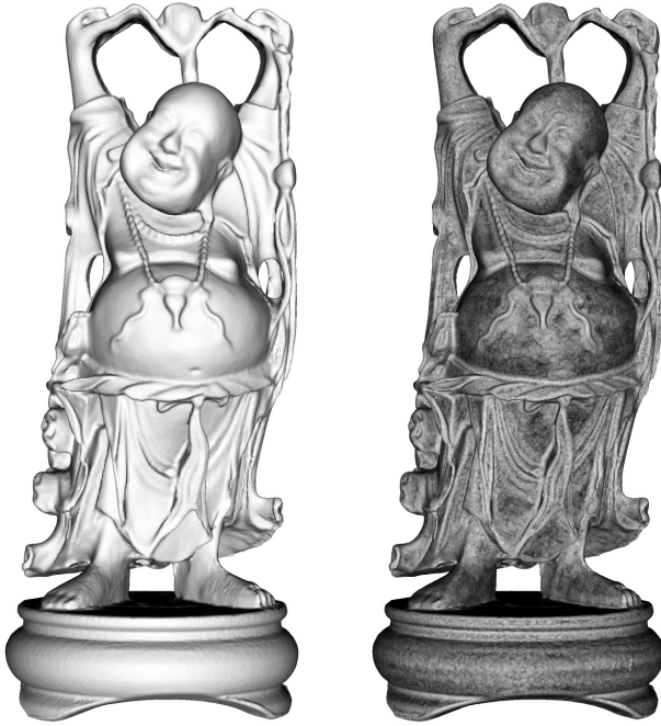
Fig. 3. Curvature indicator for the Happy Buddha model. Left: original model, right: curvature indicator (higher values are brighter)
