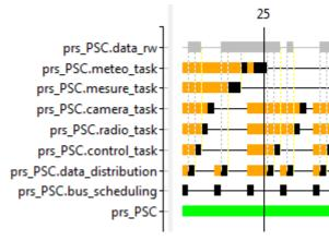
Note that the *Threads* are shown with an increasing level of priority (i.e. the bus scheduling *Thread* has the highest priority). If the PCP concurrency protocol is removed from the shared *Data* component, the "priority inversion" problem is displayed by Marzhin as follows:
