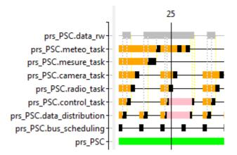
We can observe that some high priority *Threads* are postponed by low priority *Threads* that are blocking the access to the shared *Data*. The priority inversion phenomena is highlighted by the fact that the high priority *Threads* are in a "wait for resource" state
