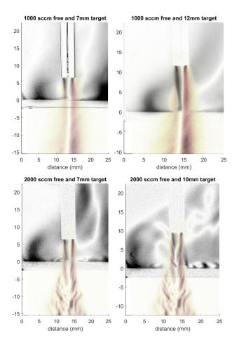
Figure 8. The comparison of the structure of flow between the freely expanding jet and the plasma jet with a glass target in front of it, for 1000 SCCM and 2000 SCCM He flow. The images were made by overlaying the relevant images of flow. The flow with a target is shown in grayscale, while the flow of the freely expanding jet is given in colour. The plasma was always on.
