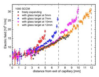
Figure 5. Electric field profiles as a function of the distance from the exit of the capillary. The measurements were taken at 30 kHz, 2 kV amplitude (4 kV<sub>pp</sub>). Glass target at different distances was used (5 mm, 7 mm, 10 mm and 12 mm) at a single He flow of 1000 SCCM. The positions of the targets are indicated by dashed lines.
