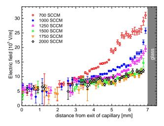
Figure 2. Electric field profiles for different flows of He as a function of the distance from the exit of the capillary. The measurements were taken at 30 kHz, 2 kV amplitude (4  $kV_{pp}$ ). Glass target was used at 7 mm distance from the exit of the capillary.
