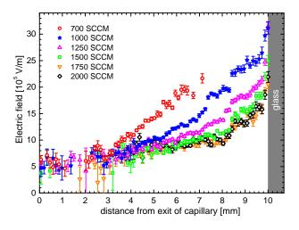
Figure 3. Electric field profiles for different flows of He as a function of the distance from the exit of the capillary. The measurements were taken at 30 kHz, 2 kV amplitude (4  $kV_{pp}$ ). Glass target was used at 10 mm distance from the exit of the capillary.
