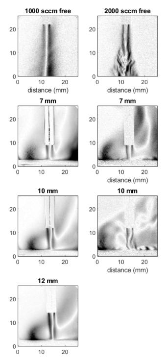
Figure 7. The visualization of the flow for two different flow speeds (1000 SCCM and 2000 SCCM) in a freely expanding jet and with a glass target at different distances. Flow visualization of freely expanding jets was shown in [26].
