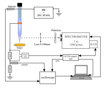
**Figure 1.** The experimental setup. Modelled after the figures in [21–24].
