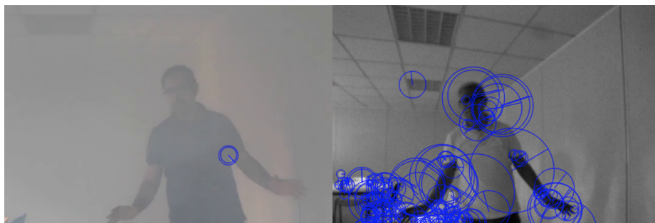
(a) Room viewed by standard RGB-camera (b) Room viewed by SWIR camera
