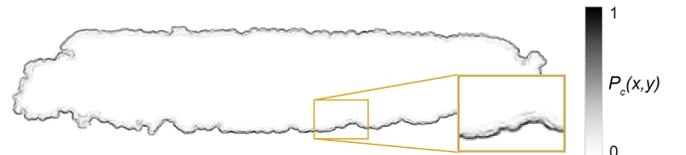
**Fig. 9.** Contour probability  $P_c(x, y)$  obtained from  $P_s(x, y)$ . The result has been scaled in the 0–1 range.
