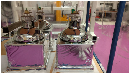
FIGURE 3: SuperNEMO optical modules with the 8-inch photomultiplier tubes on the top and the wrapped scintillators ( 256 \times 256 \times 194 mm) below.
