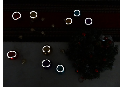
Similar objects to the template are detected in a low-contrast image with an Asplund's metric.
