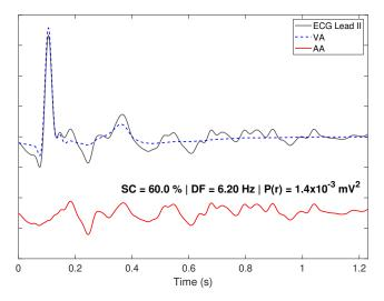
Fig. 4: Original recording, VA and AA estimates in lead II by the Löwner-based BTD of Patient P7. The AA signal was vertically shifted for clarity.
