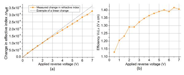
Figure 2. (a) Experimental change in the effective refractive index of the mode as a function of the DC applied reverse voltage on the phase shifter. (b) Corresponding change in the  $V\pi L\pi$  efficiency product as a function of the DC applied reverse voltage on the phase shifter.
