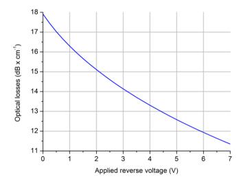
Figure 3. Optical losses in the phase shifter as a function of the DC applied reverse voltage, according to a simulation based on free carrier concentration variations.
