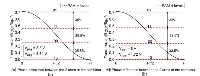
Figure 5. PAM-4 transmission levels resulting from the application on the realistic silicon MZM model of peak-to-peak voltages given by (a) the ideal lossless MZM model (8.3V on one arm and 5.34V on the other) and (b) the realistic silicon MZM model (8V on one arm and 4.72V on the other).
