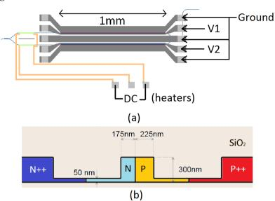
Figure 1. (a) Schematic top view of the dual-drive MZM, each phase shifter can be driven independently through coplanar travelling-wave electrodes, and thermal heaters controlled with a DC voltage can be used to tune the operating point. (b) Schematic cross section of one phase shifter, the carrier depletion regime in the PN junction is used to achieve phase modulation along the rib waveguide.
