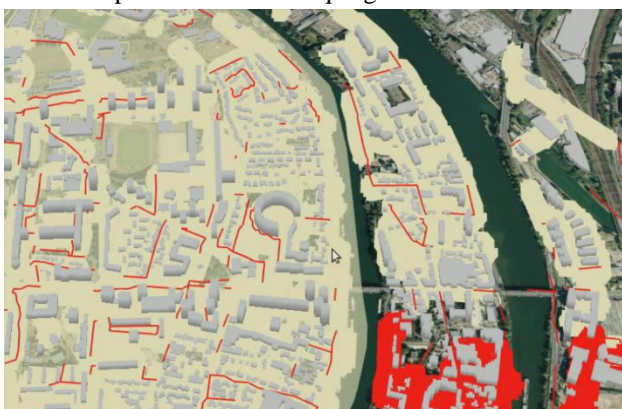
Figure 8. 3D oblique visualization of the potential impact of flood on energy network with iTowns 8 . The impacts are represented with 2D geometries put on top of 3D data.
