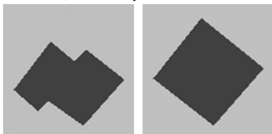
Figure 5. Two images generated from CartAGen to train a deep learning model for building generalization. The building is generalized by an agent-based process with constraints on size, granularity, squareness, and shape preservation.
