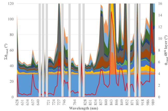
Fig. 17. Evolution of  $\Sigma\phi_{RMSD}$  versus optical monitoring wavelength for the layers 37 to 48 and overlay with the regions that are trigger point monitoring-compatible based on trinary mapping (non-greyish rectangles). The red curve represent the  $\phi_{RMSD}$  at the last layer.
