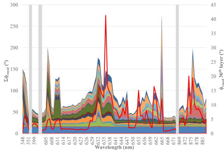
Fig. 11. Evolution of  $\Sigma\phi_{\text{RMSD}}$  at 795 nm when depositing the layers 19 to 36 for different range of optical monitoring wavelengths. The red curve represent the  $\phi_{\text{RMSD}}$  at the last layer.
