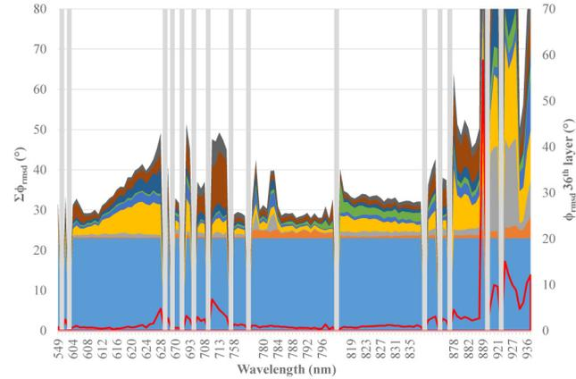
Fig. 16. Evolution of  $\Sigma\phi_{RMSD}$  versus optical monitoring wavelength for the layers 29 to 36 and overlay with the regions that are trigger point monitoring-compatible based on trinary mapping (non-greyish rectangles). The red curve represent the  $\phi_{RMSD}$  at the last layer.
