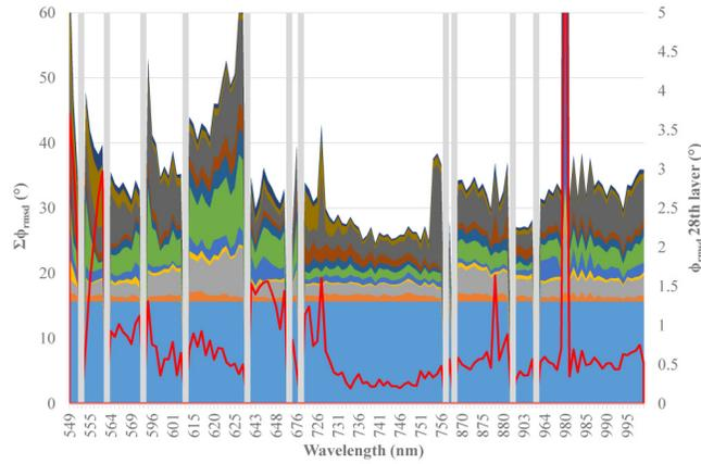
Fig. 15. Evolution of  $\Sigma\phi_{RMSD}$  versus optical monitoring wavelength for the layers 19 to 28 and overlay with the regions that are trigger point monitoring-compatible based on trinary mapping (non-greyish rectangles). The red curve represent the  $\phi_{RMSD}$  at the last layer.
