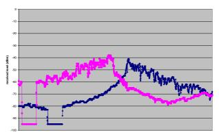
Figure 1 : Received signal level by a radio at each end of a train
