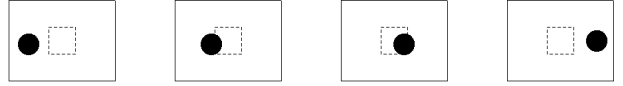
Fig. 1. Successive frames of a moving object on a white background. The local brightness of the image changes, whereas the global histogram remains constant.
