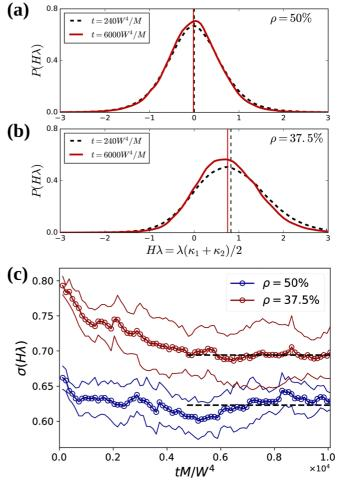
FIG. 4. [(a) and (b)] Probability distribution of the average curvature *H* rescaled with the characteristic curvature  $\lambda$  at two different times and for volume fraction  $\rho = 50\%$  and  $\rho = 37.5\%$ . (c) Temporal evolution of the standard deviation of the probability distribution depicted in (a) and (b). The symbols display the value average over ten independent simulations and the continuous lines a confidence interval.
