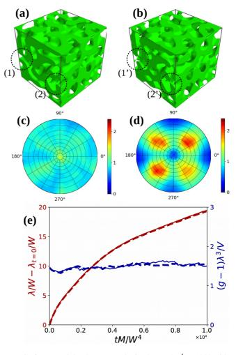
FIG. 6. [(a) and (b)] Structures obtained at  $tM/W^4 = 1200$  without (a) and with (b) interface anisotropy. [(c) and (d)] Density of surface normal without (c) and with (d) interface anisotropy. (e) Time evolution of the characteristic length scale and rescaled connectivity for both isotropic (continuous lines) and anisotropic structures (dash lines).
