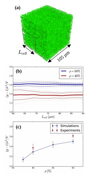
FIG. 7. (a) Tomographic imaging of a microporous FeCr sample with volume fraction 50% obtained from liquid metal dealloying [51]. (b) Rescaled connectivity as a function of the size of the analyzed volume (see text for explanations). (c) Comparison of the average connectivity with numerical results.
