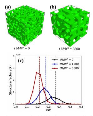
FIG. 1. (a) Example of initial microstructure considered for volume fraction  $\rho = 50\%$ . (b) Coarsened structure obtained at  $tM/W^4 = 3600$ . (c) Spherically averaged structure factors obtained from three different configurations along a simulation and the corresponding values of  $k_0$  shown with dash lines (see text for explanations).
