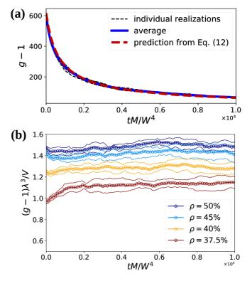
FIG. 5. (a) Time evolution of the connectivity obtained for  $\rho = 50\%$ . (b) Rescale connectivity as a function of time for different volume fraction. The continuous lines represent confidence interval of one standard deviation.
