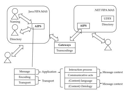
**Figure 7.** Foundation for the Intelligent Physical Agent (FIPA) specifies multi-agent systems (MAS) interaction using specifications for an Agent Interaction Protocol Suite (AIPS) and MAS platform [107].
