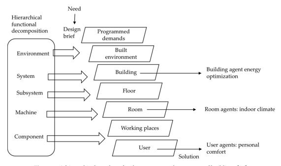
Figure 4. A hierarchical ontology for the energy supply structure of buildings [16].
