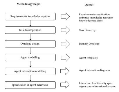
**Figure 6.** Agent design methodology stages and their output used during the design of the PEDA (Protection Engineering Diagnostic Agents) system [110].
