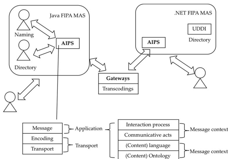
**Figure 7.** Foundation for the Intelligent Physical Agent (FIPA) specifies multi-agent systems (MAS) interaction using specifications for an Agent Interaction Protocol Suite (AIPS) and MAS platform [107].
