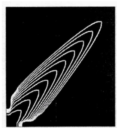
Figure 5: Dendritic growing of a partially faceted crystal from a pure liquid (phase-field numerical simulation) (Debierre et al., 2003).
