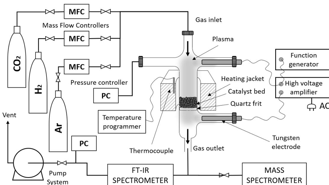
Fig. 1 Scheme of plasma-catalytic set-up used for the evaluation of the performance of prepared materials.
