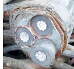
Fig. 2. Section of multiple aluminum beams cable
