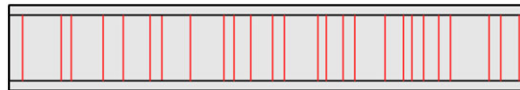
FIGURE 19 Schematic representation of the crack location for a specimen tested at 500 \text{ mm min}^{-1}
