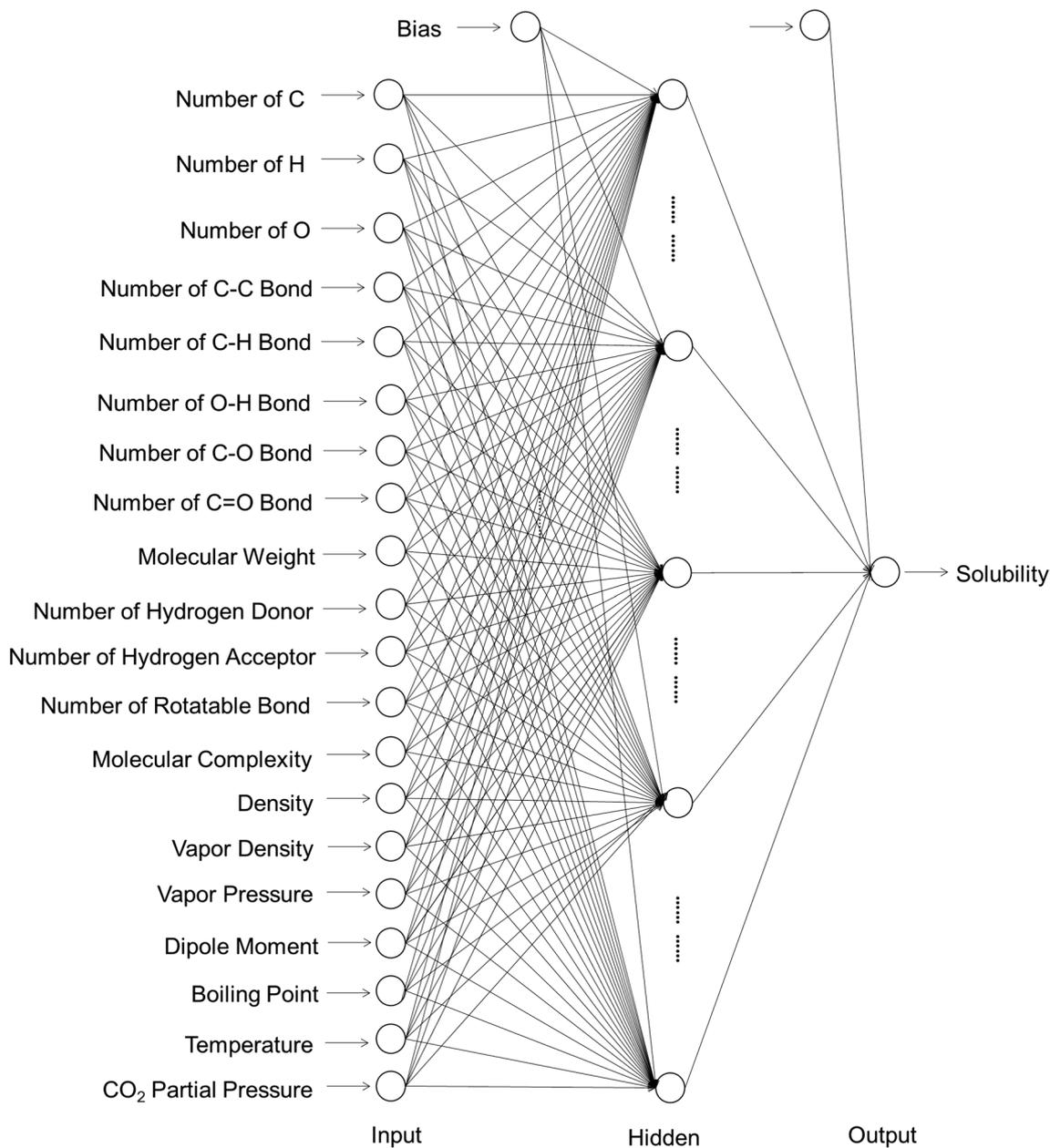
**Fig.1** Structure of the back-propagation neural network (BPNN) developed in this study, with the input, hidden, and output layers. The empty circles represent the neurons of the artificial neural network
