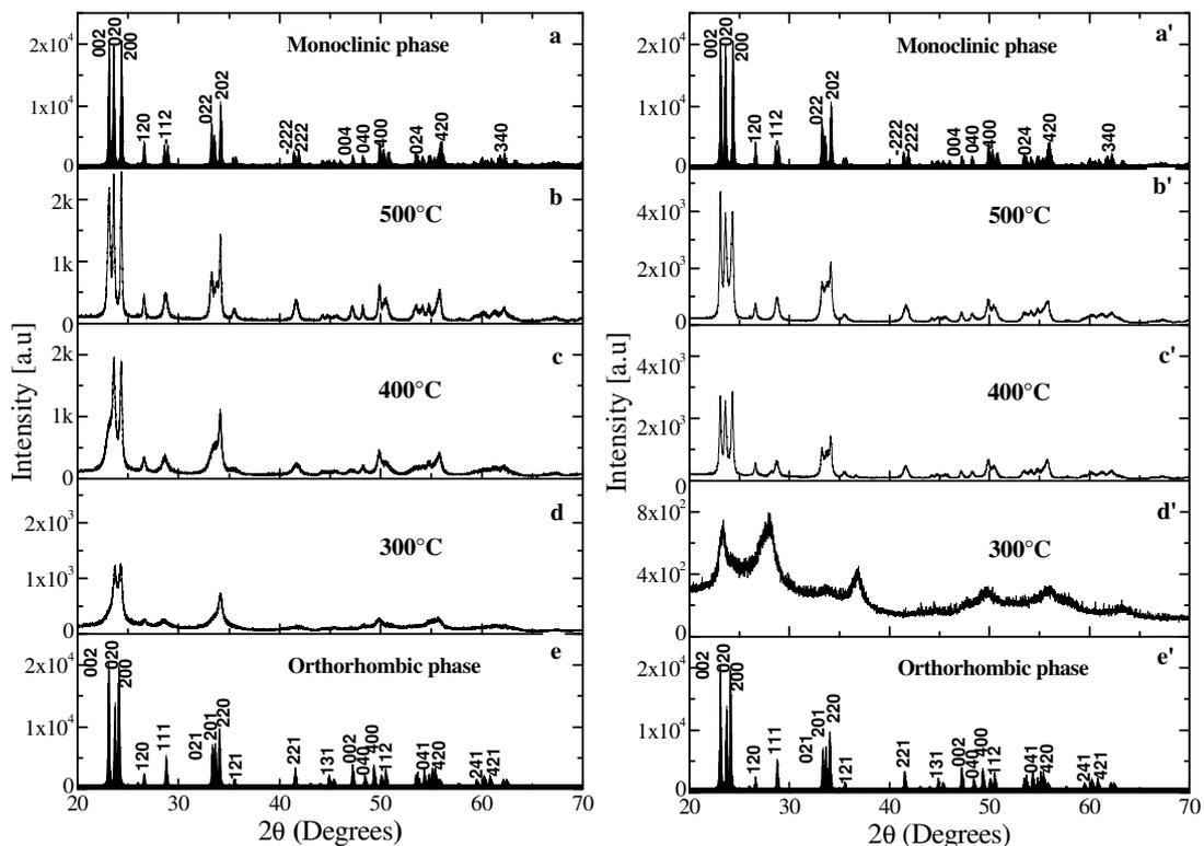
**Fig. 2.** X-Ray Diffraction patterns of  $\text{WO}_3$  powders, (b to d) for NP and (b' to d') for PS calcined at different temperatures compared to the monoclinic (a,a')/orthorhombic (e,e') simulated ICSD data sheets
