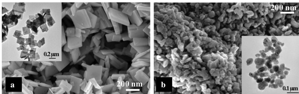
**Fig. 3.** SEM images of  $\text{WO}_3$  powders obtained by a) the NP synthesis method and b) the PS synthesis method after calcination at  $500^\circ\text{C}$ . Inserts are TEM images of the same samples
