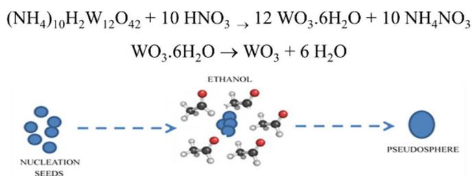
**Fig. 5.** Equation and schematic mechanism of PS formation
