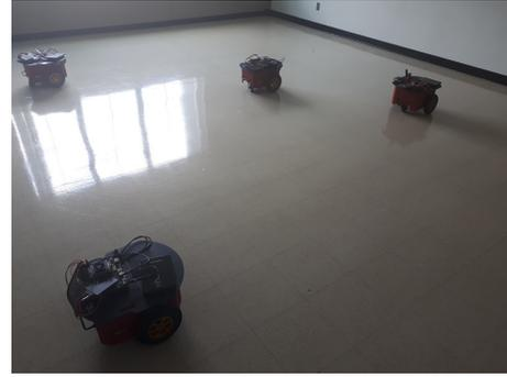
Fig. 6: Initial position of a fleet of four Pioneer 3-DX mobile robots
