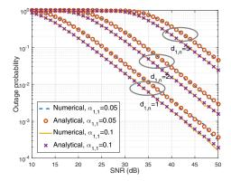
Fig. 6: The outage probability of the near user vs SNR with different  $\alpha_{1,n}$  ( $\gamma_{1,n}=1$ )
